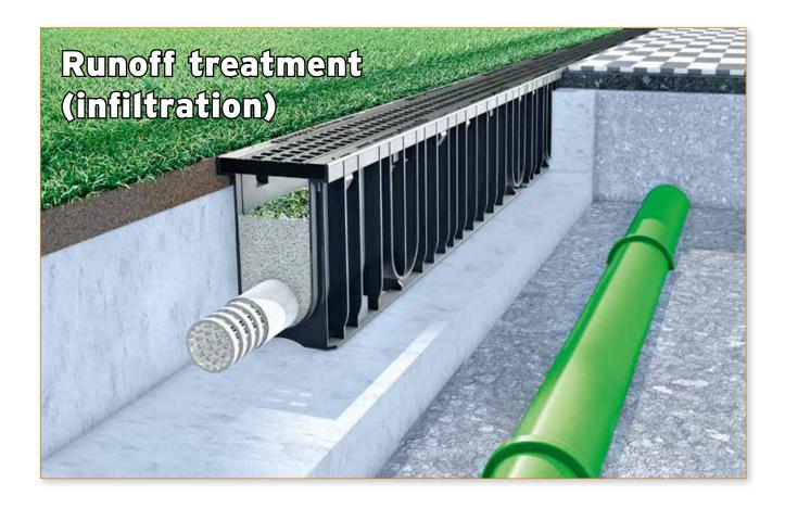
**SPORTFIX**<sup>®</sup>CLEAN 100 Type 020 with GUGI mesh grating and infiltration pipe in combination with **CARBOTEC**<sup>®</sup>60 substratum for drainage and treatment of storm water runoff from artificial turf pitches.
